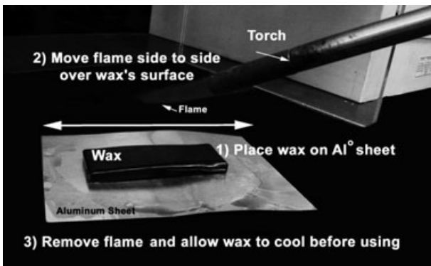
FIG. 6—To remove heavy scratches, gently heat wax surface with a torch and allow to cool.
