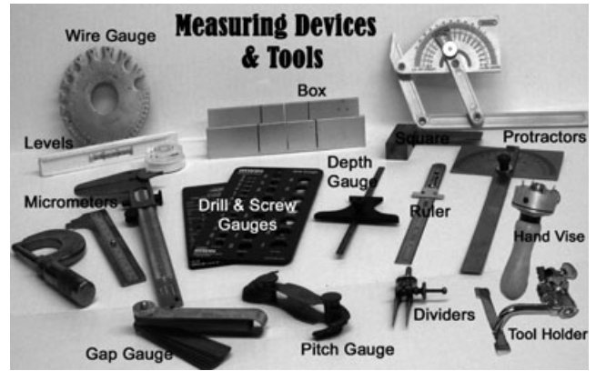
FIG. 4—An assortment of devices used to study questioned tool marks for the purpose of preparing tool mark standards in the same or similar manner as the questioned tool marks were made.
