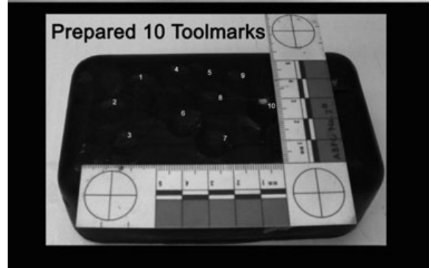
FIG. 10—A ball peen hammer striking the surface of a block of soft sculpting wax at an angle of 23°. Ten tool mark standards were produced for comparison purposes. All ten exhibited the same class characteristics, damage marks, and patterns.
